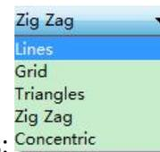
The drop down menu for the support mode is shown as follows: , Users can set different forms of support according to different models, so that support can be conveniently removed and better support and model contact surfaces can be obtained. Among them, lines, grid and zig zag shape support are mostly to be choose.
