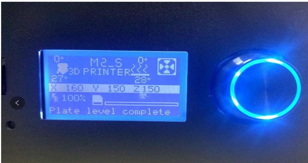
After adjust, if the gap between the nozzle and platform is not suitable, please repeat to adjust each point.
